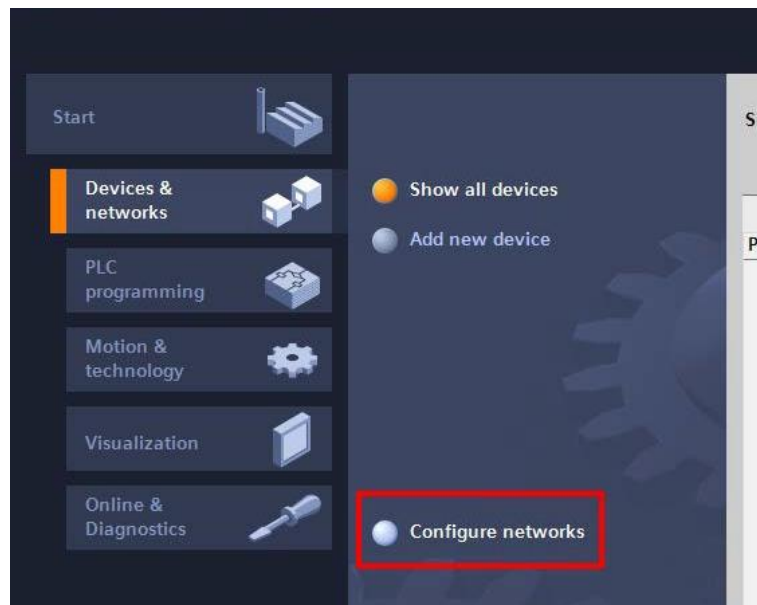
Figure 105: TIA - Configure Networks
